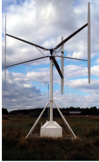
Figure 3.4. The 12 kW turbine, designed and built by the Division of Electricity at Uppsala University. The turbine is equipped with load cells used for the force measurements [14].
