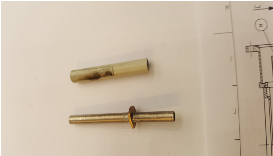
Figure 3.4: The damaged G2 tube and insulator
