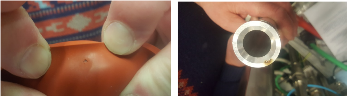
Figure 3.8: Arcing damage at the inside of the hose and the connector
