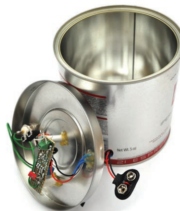
Figure 1. The radiation detector that the pupils assembled and used in their measurements. Photo courtesy of Mats Kamsten at Uppsala University.
