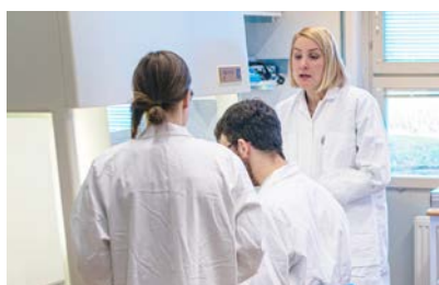
The laminar flow cabinet in which the course participants work is equipped with an extractor fan. This means that any airborne particles formed during handling or in the event of an accident are sucked into the cabinet and caught in the filter.
