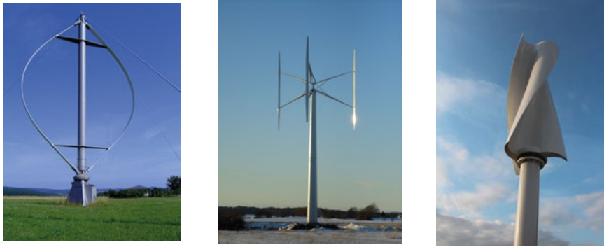
Figure 1.1. Left : Curved-bladed Darrieus wind turbine [7], middle : Straight-bladed Darrieus wind turbine (picture from Vertical Wind AB), right : Savonius wind turbine [8]
