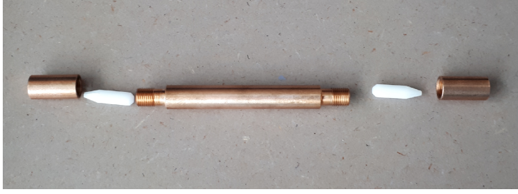
Figure 4: Cu cylinder (ferrule) and the tefflon fixtures.
