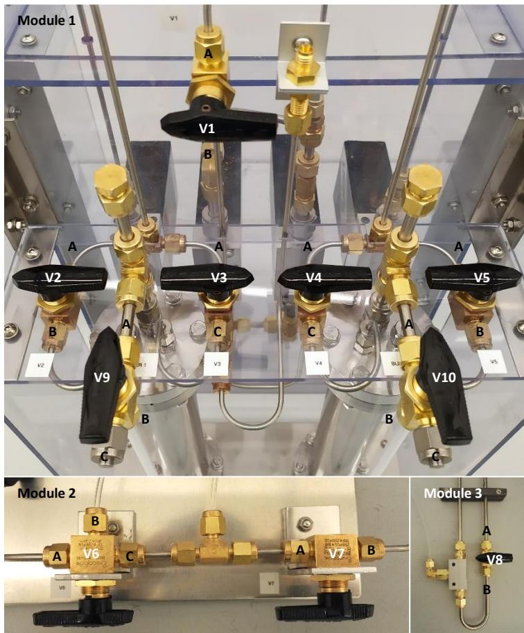
Figure S23: The *dSVA* control and sight glass valves (V1-V10) with the ports (A, B and C) labelled with reference to the *operational states* listed in
