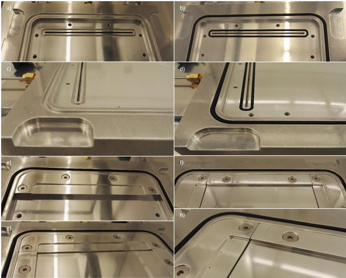
Figure S9: The SVA chamber in various stages of assembly and from different angles. To the chamber body (a and c) are added the o-rings (b and d), the gas distribution nozzles (e), and the chamber insert (f-h).
