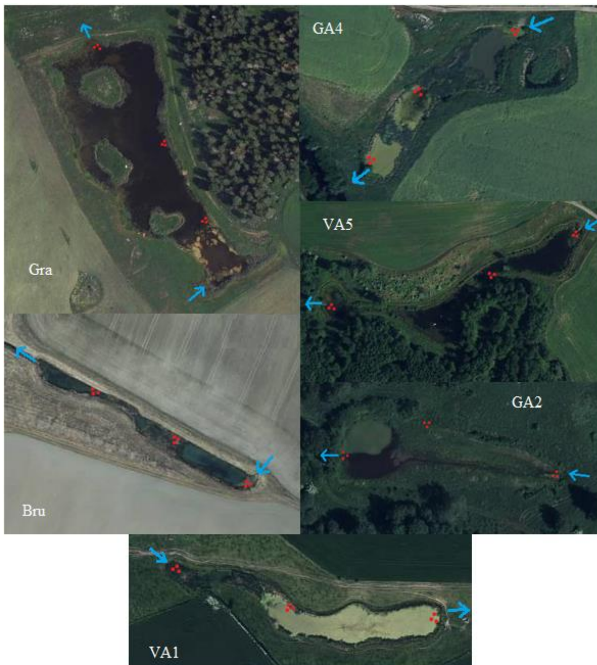
Figure 3. Floating chamber locations in six of the CWs where the red dots symbolize the chambers, and the blue arrows marks the in- and the outflow. The three chambers in Bru are placed with some distance to the outlet due to vegetation hindering the deployment. In Gra the water near the inlet contained a large amount of water vegetation and the other chambers were placed at a free water surface, therefore the placement further down the wetland.
