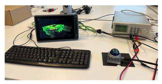
Figure 4.9: The CCpilot X900 display computer to left presenting point cloud data from the Mid-360 LiDAR to the right.
