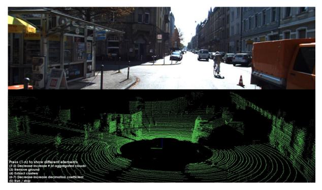
Figure 2.1: A camera view at the top and the LiDAR view at the bottom [5].
