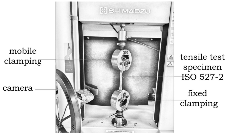
Fig. 4 Unidirectional testing machine equipment in the Ångström Laboratory, Uppsala University
