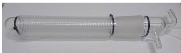
Fig. 3 The coiled Teflon tube around the water-cooled condenser is used for the photodimerization reaction of dienes. The reaction was run at ~7 °C. The starting experimental solutions containing diene and 1,1-dinaphthylmethanone mixture were transferred into the Teflon tube and both ends were sealed with rubber septa
