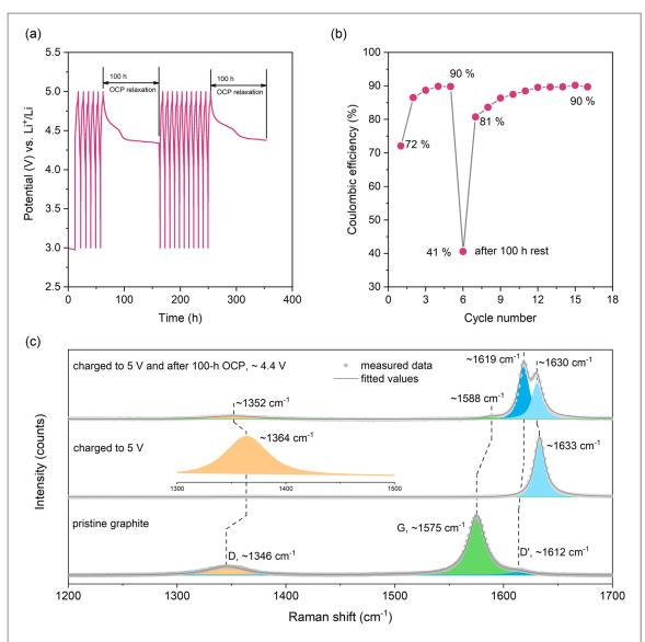
Figure 5. Tracking self-discharge of a DIB charged to  $5\,\mathrm{V}$  and allowed to rest for a  $100\,\mathrm{h}$  (a) the chronopotentiograms with OCP relaxations after the  $5\,\mathrm{th}$  and  $18\,\mathrm{th}$  cycles (b) the coulombic efficiency for the cycles shown in (a), (c) the Raman spectra for pristine graphite, FSI-intercalated graphite at  $5\,\mathrm{V}$ , and graphite electrode charged to  $5\,\mathrm{V}$  and after a  $100\,\mathrm{h}$ -OCP rest.
