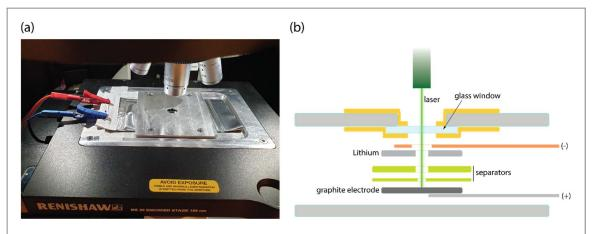
**Figure 1.** Monitoring structural changes in graphite electrode using *in situ* Raman spectroscopy: (a) a picture showing the pouch cell designed for *in situ* Raman scattering measurements, and (b) a schematic illustration showing the arrangement of electrodes and separators in the pouch cell in (a).
