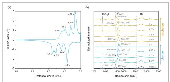
**Figure 3.** Monitoring structural changes in graphite electrode using *in situ* Raman spectroscopy: (a) the differential galvanostatic plots showing the charge–discharge peaks associated with GIC phase transitions, and (b) the *in situ* Raman spectra measured on the different GIC phases indicated by the charge–discharge peaks in (a).
