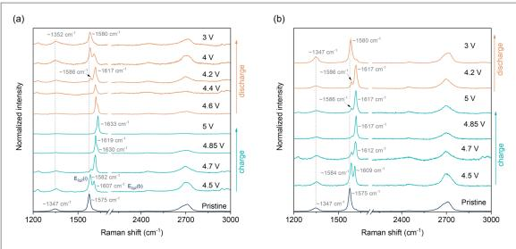
**Figure 4.** Raman spectra measured *ex situ* on graphite electrodes during charge and discharge processes after self-discharge relaxations at OCP over (a) < 10 h, and (b)  $\sim$ 1 week.
