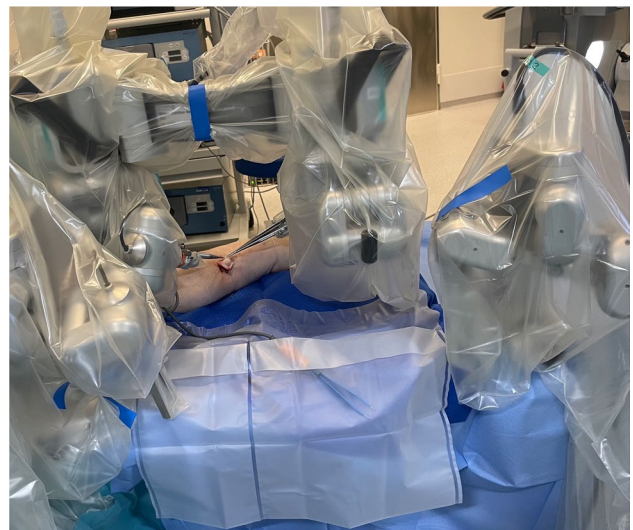
Fig. 3 After vessel preparation, the robot was positioned in place, and the microsurgical instruments were mounted to the robot arms. During setup, the surgical field was protected with a moist gauze
