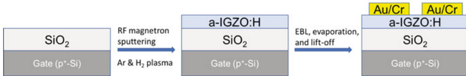
Figure 3.1 Schematic of the main fabrication processes of IGZO:H-TFTs.
