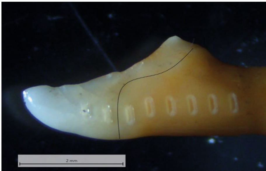
Figure 5. Ablated cyprinid tooth, with the EDJ, indicated with a dotted line. Ablations from left to right; first two targeting only enameloid, with valid Sr ratios; the third located on the EDJ, with Sr ratios reflecting a mixture of enameloid and dentine Sr ratios. The fourth to eight ablations targeting dentine only, Sr values reflecting a mixture of the Sr ratios of the dentine with an unknown admixture of depositional environmental Sr ratios. Photo B. Krooks
