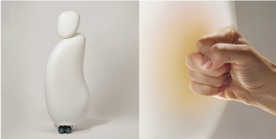
Figure 3: Fighting Baymax: A robot sparring partner that motivates practitioners to exert more force
