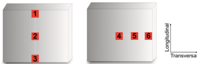
Figure 4.3. The six measurement sites for synchrotron diffraction. The build direction is in the longitudinal direction.
