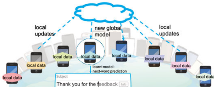
Figure 2.1. An example application of FL for the task of next-word prediction on mobile phones [27]. To preserve the privacy of the text data and to reduce strain on the network, we seek to train a predictor in a distributed fashion, rather than sending the raw local data to a central server.
