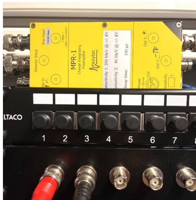
Figure 6. The Mesytec MPR-1 preamplifier (yellow box) installed in the NESSA inner bunker. The pre-amp is kept close to the neutron generator to keep the cable length to the fission chamber as short as possible.
