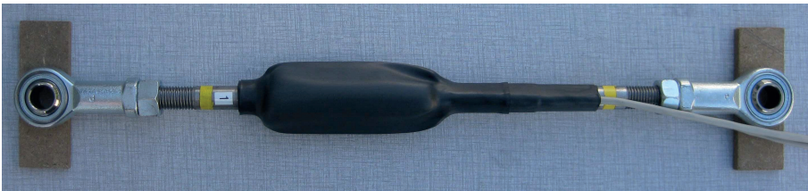
Figure 6.7. The stator was secured radially with four 16mm metal rods. Figure 6.4 shows the position of the rods. Each rod was equipped with four strain gauges in a wheatstone bridge.
