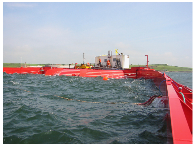
Fig. 4. The Wave Dragon deployed and tested in the sea [20].
