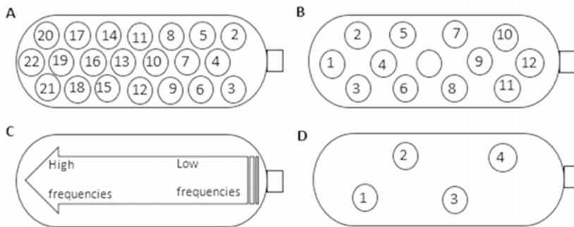
Figure 12. (A) Electrode from Cochlear (Lane Cove, NSW, Australia), dimension: 3 x 8.5 mm. (B) Electrode from MED-EL (Innsbruck, Austria), dimension: 3 x 5 mm. (C) Theoretical frequency order on the implant. (D) ABI placing system from MED-EL dimension: 3 x 5 mm.
