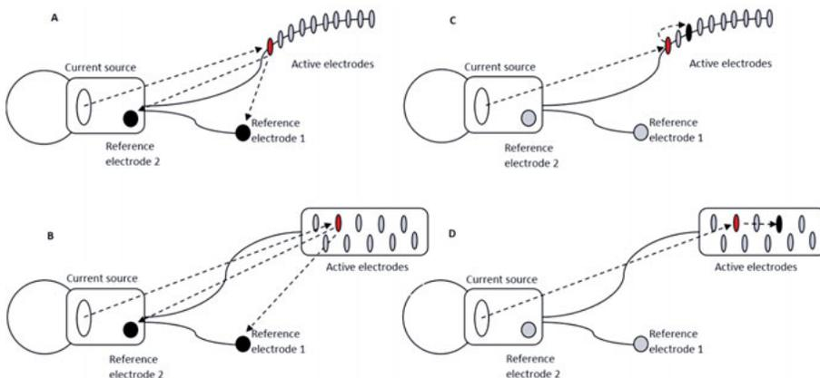
*Figure 4.* Electrodes colored in red represent the stimulated electrode and electrodes colored in black the ground/reference electrode. (A) monopolar mode on a CI (B) monopolar mode on an ABI (C) bipolar mode on a CI, BP+1 (D) bipolar mode on an ABI, BP+5.
