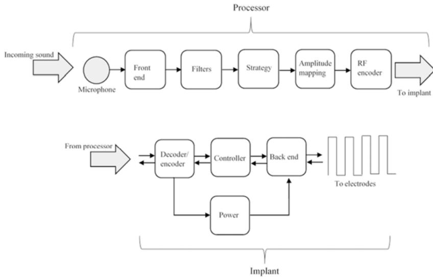
Figure 3. The principles of a sound processor and an implant. Modified illustration from Clark (2003).
