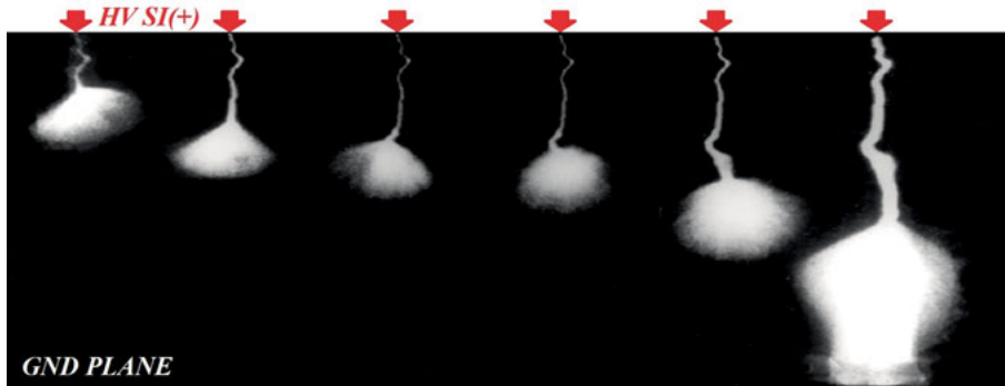
Figure 3. Frame photograph from a 10 m cone-to-plane electrode configuration tested with positive voltage switching impulses 500/10000 \mu\text{s} (adapted from [26] with permission from the editor).
