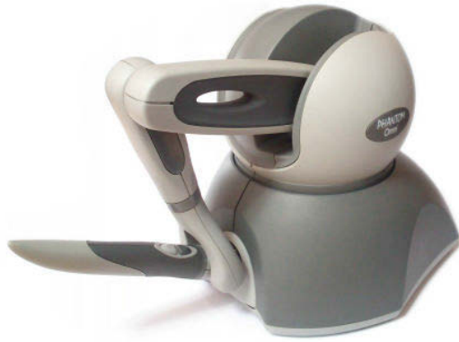
Figure 4.10. A Sensable Phantom Omni haptic device with six degrees of freedom (6-DoF) input and three degrees of freedom (3-DoF) output.
