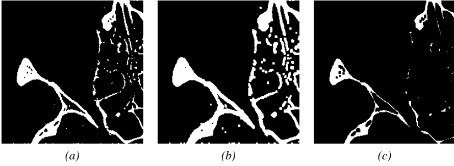
Figure 3.5. Fundamental binary mathematical morphology operations performed with a 26-connected 3D structuring element: (a) original binary image; (b) dilation; (c) erosion.
